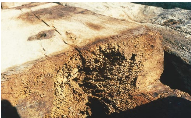
Figure 10: Death watch beetle attack in 15th Century church timbers
