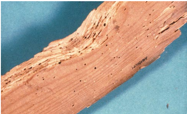
Figure 9: Common furniture beetle attack, showing a number of flight holes
