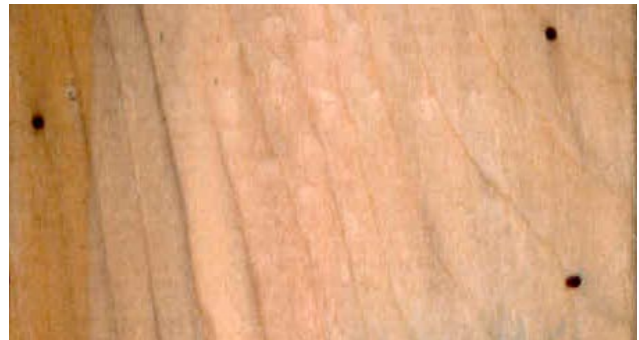
Figure 7: Typical dark rimmed bore holes of ambrosia beetle damage in sapwood
